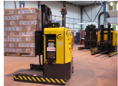
Figure 2: A forklift-based AMR, like this one produced by TUDOR, is capable of autonomously finding pallets on a warehouse floor, and carrying them to their destination. Image from Wikipedia: https://commons.wikimedia.org/w/index.php?curid=7838942
